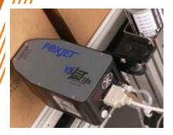
The VxSeries 18x print head is available in 1" and 2" print heights. Its durable diecast aluminum housing makes it ideal for challenging industrial environments. The print head can be daisy chained with up to 3 other VxSeries 18x print heads, allowing it to print large logos or large multi-lined alphanumeric text messages.
